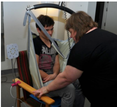
ER AIS: Ergonomic Aiding Seat enables a nurse to correctly position a patient by monitoring pressure data from the wheelchair seat, which is displayed on the LED display at left.
